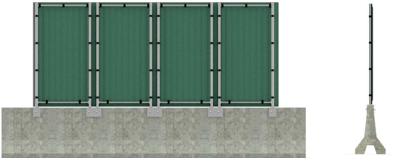
EXAMPLE OF INSTALLATION ON A NEW JERSEY
